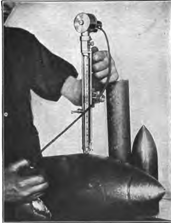
Fig. 189. Testing Hardness of Projectiles Courtesy of Shore Instrument Company, New York City
